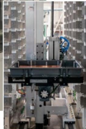
Transport shuttle with box and inner layer
